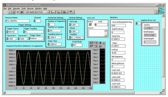
This VI demonstrates how to use some of the basic components of the AqDx Acqiris Digitizer Driver. It finds and initializes a digitizer, sets the basic parameters according to the controls on the front panel, and then acquires one waveform. Note that the front panel controls should be set to their desired values before the VI is run.
