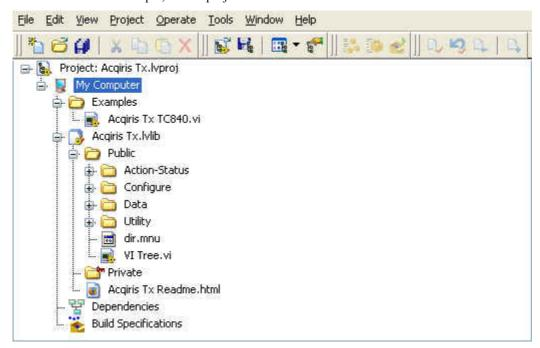
The Example folder contains ready to use potential starting points for your own programs. Individual library functions can be found at the Public level or in one of the 4 categories shown. Query functions are in the Utility folder. The block diagram of the VI Tree.vi can be used to access individual functions. It allows quick and easy access to all needed vi's.
