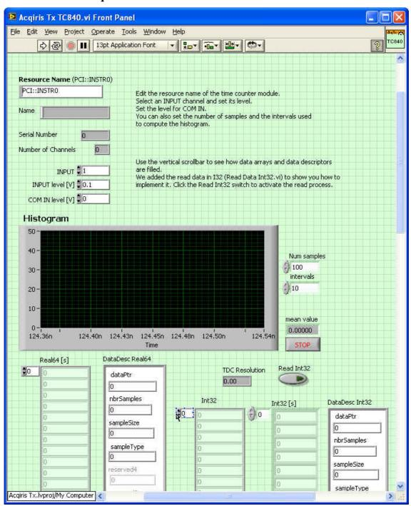
This VI demonstrates how to use a TC840 Time Counter. It finds and initializes an instrument, sets the basic parameters according to the controls on the front panel, and then acquires and accumulates data as the user requests. Note that the front panel controls should be set to their desired values before the VI is run.
