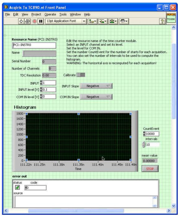
This VI demonstrates how to use a TC890 Time Counter. It finds and initializes an instrument, sets the basic parameters according to the controls on the front panel, and then acquires and accumulates data on the common and the chosen channel as the user requests. Note that the front panel controls should be set to their desired values before the VI is run.
