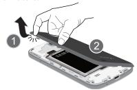
**Note:** The battery cover is flexible. Take care to avoid bending or twisting the cover when removing and installing to prevent damage to the cover.
