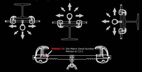
Climbtech anchors are manufactured to meet the requirements of ANSI z359 and EN795: 2012 Type B. They also exceed the requirements for anchors specified in BS ISO 22846 Personal equipment for protection against falls – Rope access systems, and BS 7985 Code of practice for the use of rope access methods for industrial purposes – recommendations and guidance supplementary to BS ISO 22846. Therefore, these anchorage connectors are suitable and appropriate for rope access / suspension work.
