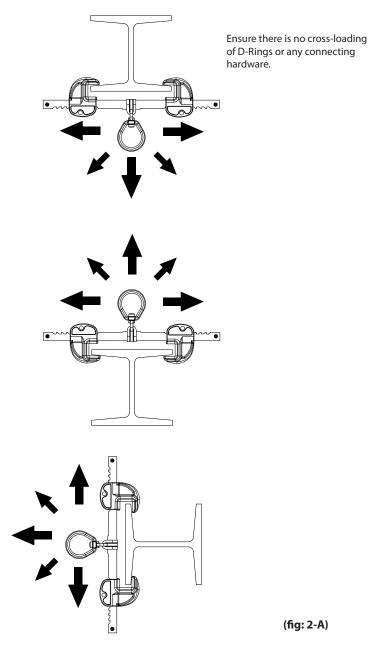
Placement at or below a user's working height requires integration of a compatible ANSI 359.1 shock-absorbing lanyard that does not allow the user to extend more than 6 feet (1.8m) (in any direction) from the anchorage connector before the shock absorber is activated. The beam anchor must be attached to the I-Beam flange facing the user (top flange is above , bottom flange is below, etc).
