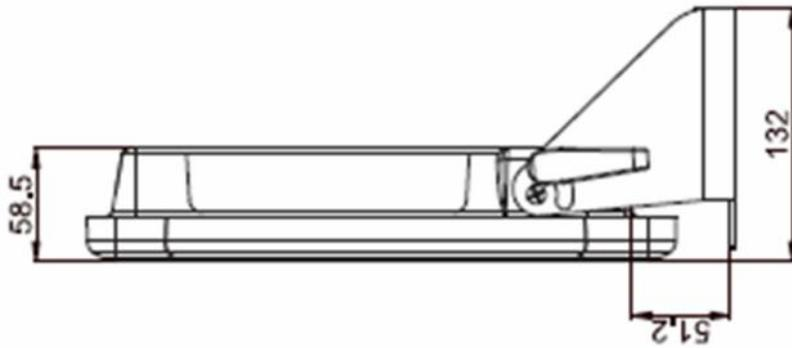
5.2 MILRM20L100-A2 Mechanical Drawings (With Mounting Bracket) Continued:
