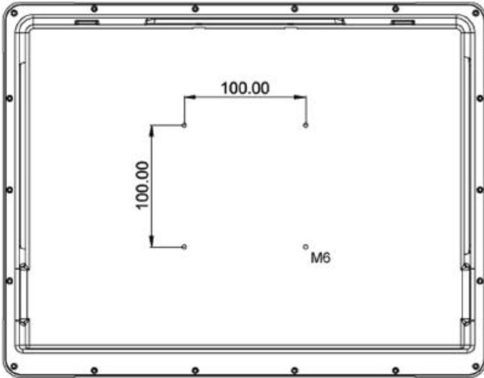
5.2 MILRM20L100-A2 Mechanical Drawings (With Mounting Bracket):
