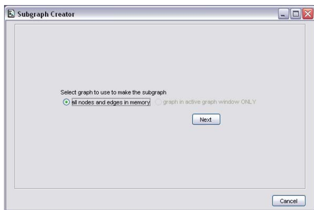
Figure 21. Subgraph Creator dialog's first screen. The graph in active graph window ONLY option is disabled because no graph was open in FCModeler when the Subgraph Creator was started.
