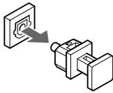
The DV-SP1000/DV-SP1000E's optical digital output sockets have dust caps for keeping out dust and dirt when they're not in use. Remove the cap before inserting an optical plug, and push the plug in all the way to make a good connection. Keep the dust cap in a safe place for future use.
