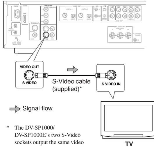
Audio connection not shown here. Make a suitable audio connection to your TV, AV receiver, or amp.
