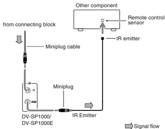
Only remote controller signals received by the DV-SP1000/DV-SP1000E's IR IN are fed through to the IR OUT. Signals picked up by the DV-SP1000/DV-SP1000E's remote control sensor are not.
