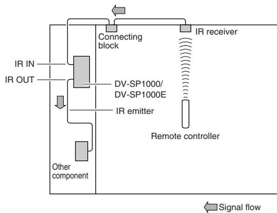
Connect the IR emitter to the DV-SP1000/DV-SP1000E's IR OUT, and place the IR emitter in front of the other AV component's remote control sensor (usually located on its front panel), as shown below. See the instructions supplied with the IR emitter.
