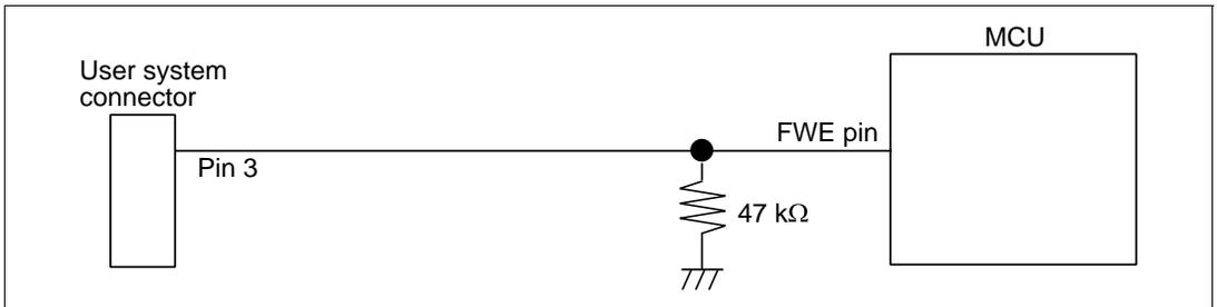
**Figure 1.5 Connection of Emulator and FWE Pin**
