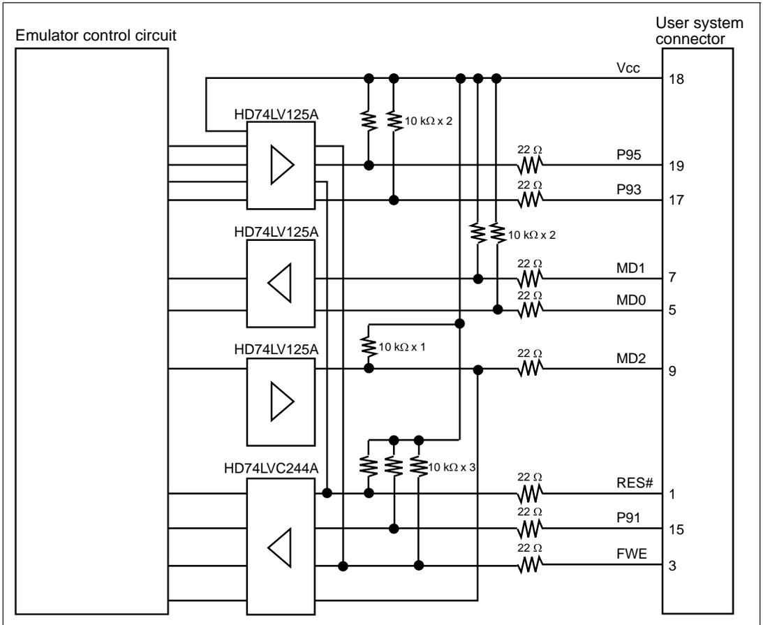
**Figure 1.8 Interface Circuit in the Emulator (Reference)**
