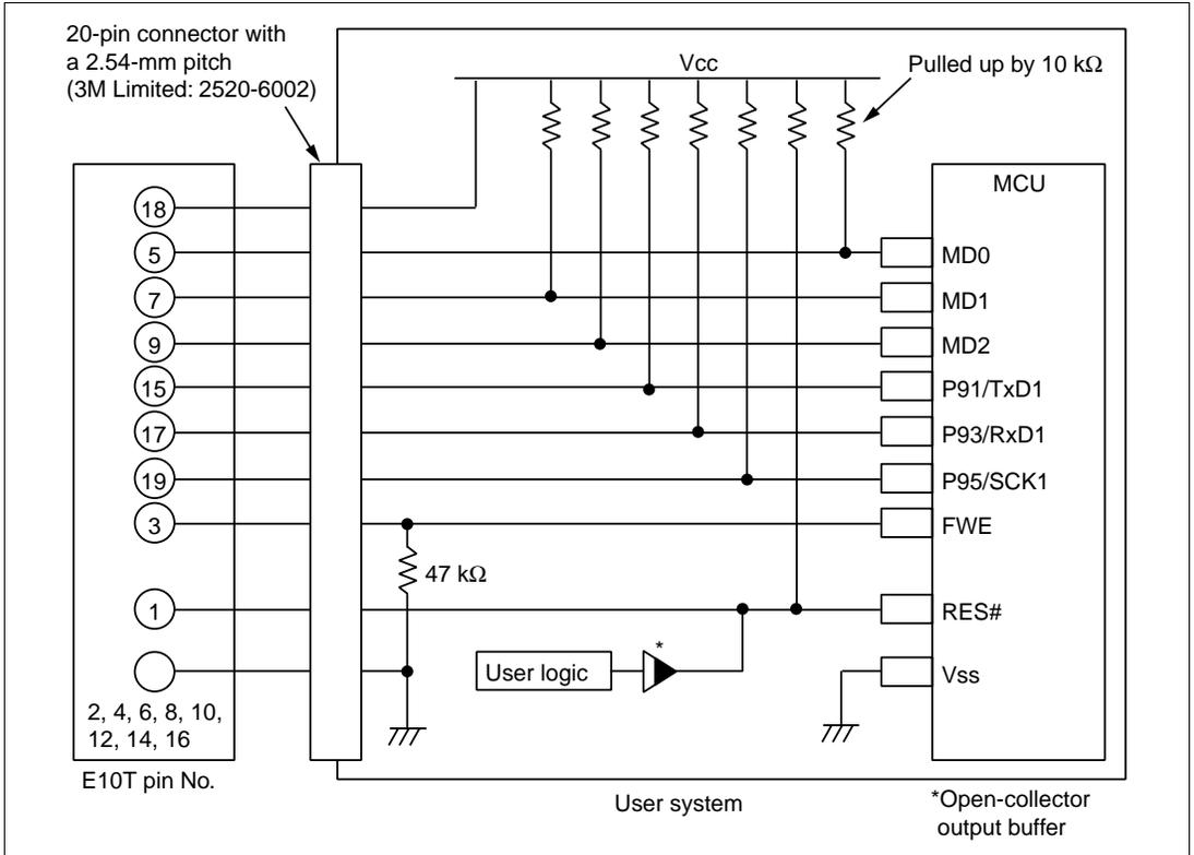
**Figure 1.3 Example of Emulator Connection (Mode 7)**
