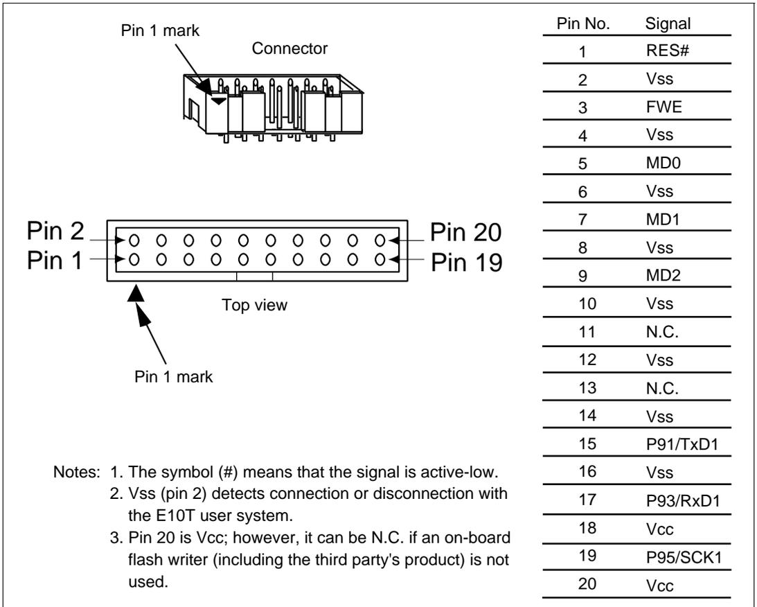
**Figure 1.2 Pin Assignments of the Connector**
