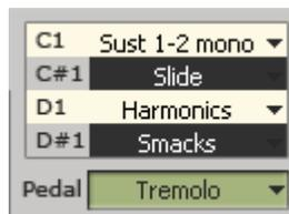
Any of 4 keys of Left Repeat zone (C1-D#1) as well as Sustain Pedal can be also used to temporarily switch the Main zone to new sound/articulation previously chosen in the respective combo box. Pressing the appropriate key or the sustain pedal switches the Effect on, while releasing the key/pedal reverts Main zone to the original sound/articulation. You can use various Key/Pedal switch FX's at a time.
