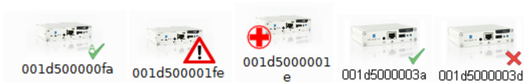
Icons left-to-right: auto-discovered, safe mode, recovery mode, manually added and unreachable
