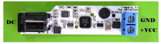
First, insert each wire of your LED string (or any other device) in the corresponding hole in the terminal block and then tighten the screw into place.
