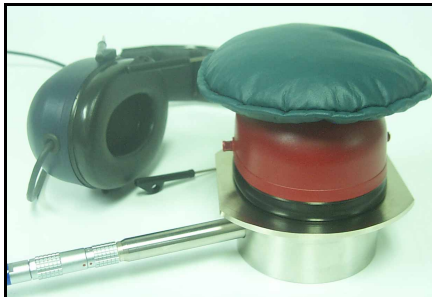
Figure 3-8 Sennheiser earphone and weight being installed on AEC101
