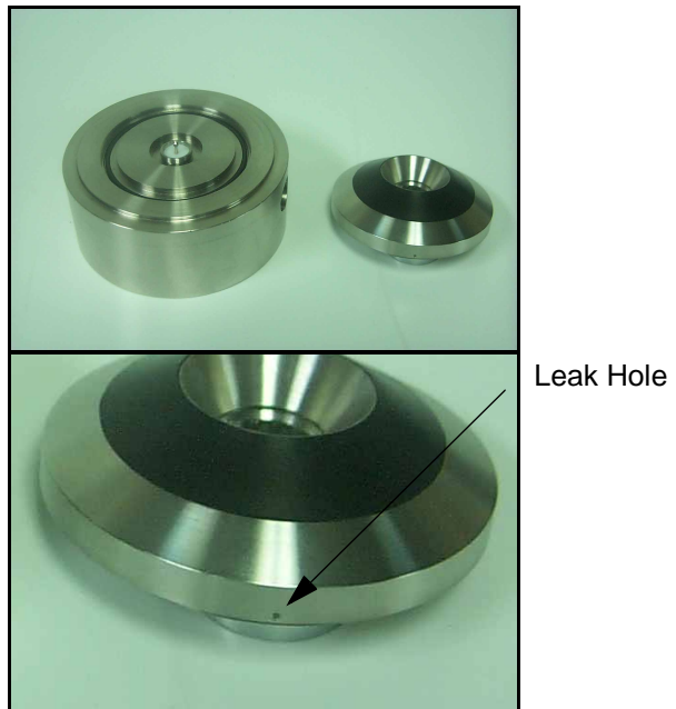
Figure 2-1 AEC101 with coupler, leak hole
