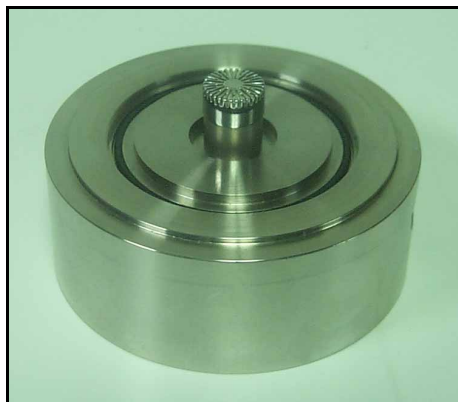
Figure 2-2 Microphone installed on AEC101
