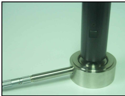
Figure 2-4 Installing the CAL250 on AEC101
