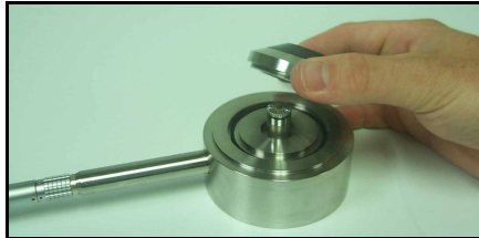
Figure 3-5 Coupler being installed on AEC101
