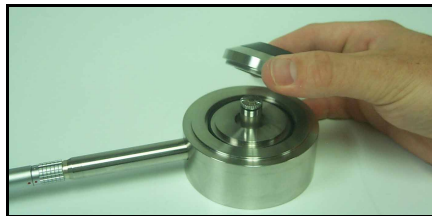
Figure 3-1 Coupler being installed on AEC101
