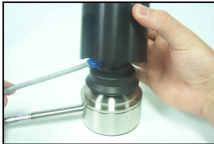
Figure 3-3 Retainer ring being installed on AEC101
