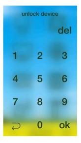
If the lock mode is enabled, the screen will ask for the password every time that changes from standby to active mode. If the lock mode is disabled, the Smart Touch can be activated and therefore used by anyone just by clicking on the screen.
