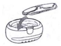
**4.** After 3 minutes, the cleaning automatically stops and the Red light turns off. Or press OFF to stop. For another cleaning cycle, just repeat above process.
