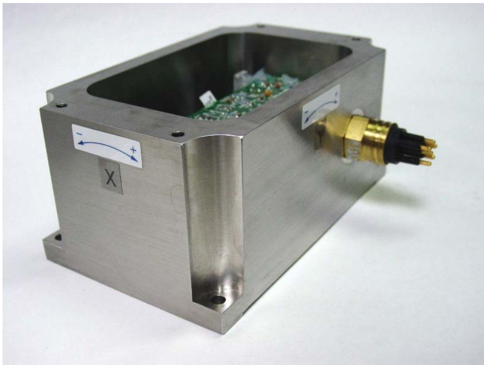
Figure 2. Biaxial DeepWater 420 tiltmeter showing X tilt direction and polarities. This direction is the same as “transverse” tilt in uniaxial versions of the tiltmeter.
