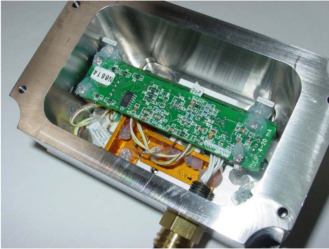
Figure 10. Interior of biaxial DeepWater 420 showing gold sensor assemblies, circuitry and silicone rubber strain relief on fasteners.
