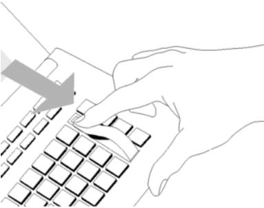
All function keys are given standard frequently-used functions. You can insert the appropriate label strips alongside the function key line. You can find this on the sheet supplied.
