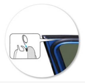
• Ensure door seal positioned as shown.
