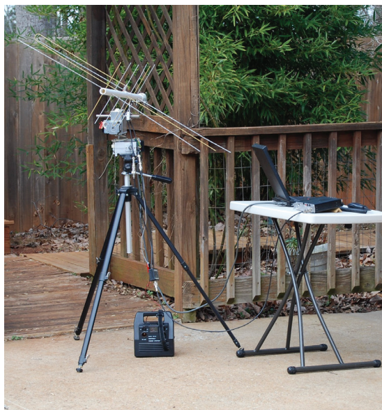
Figure 1 Complete Ground Station Using CNCTRK System
