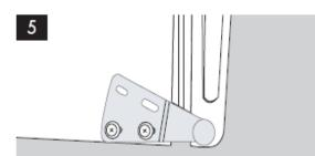
Remove the two screws from top bracket and replace on the other side. You will need to first remove the plastic caps from the other side.
