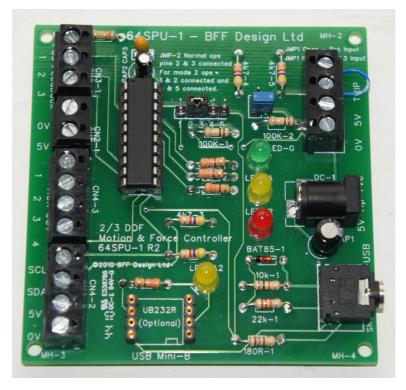
The 64SPU-1 Signal Processor Unit is designed for use with the BFF PID Servo Controller software as part of a DIY motion platform closed loop position feedback PID servo control system. V2.6beta96 or later of the PID Servo Controller (V2.6beta963 for Firmware B support) and v2.6 or later of the BFF Motion Driver software are required. For details of a typical overall system arrangement see the illustrative System Wiring Diagram at the end of this document.
