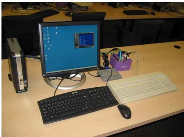
Figure 1 – PC Development environment and Diamond Systems pc-104 board target system showing picture-in-picture target system console.
