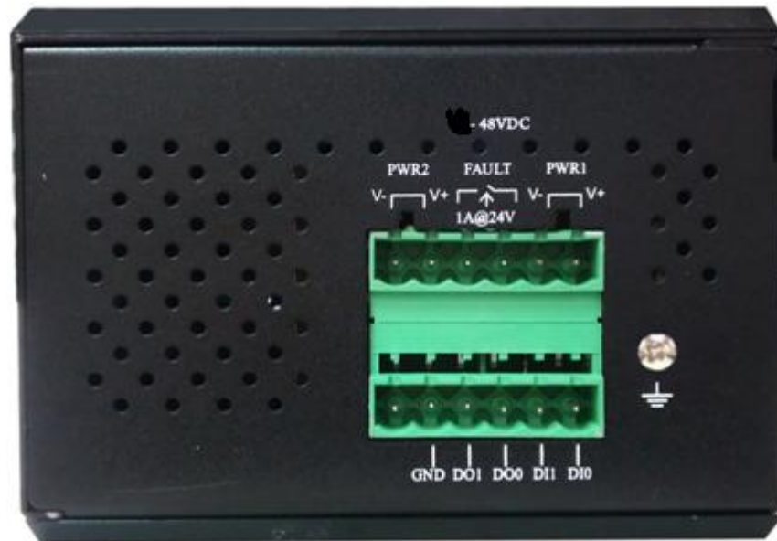
Top Panel of the industrial switch
