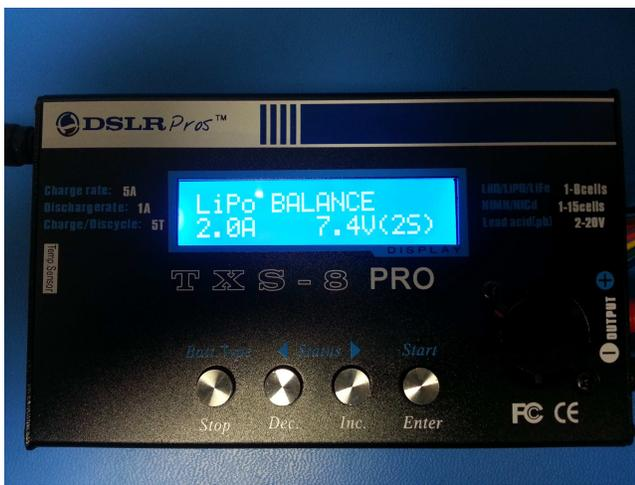
It is recommended that you use the Balance(BAL) setting when charging LiPo batteries.
