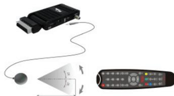
The coaxial cable, with satellite signal, must be connected to the "IF IN" connector. The "TV SCART" connector must be connected to the TV set.
