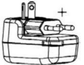
2. Press the release button that frees the North American plug from its embedded position. Continue to push the North American plug upward until it locks into a 90-degree position.
