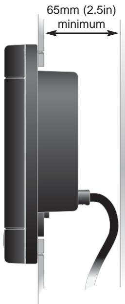
Fig 4.2 - Clearance Required Behind Bulkhead
