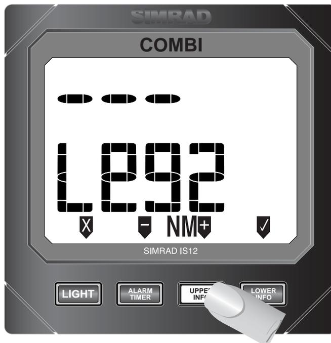
*Fig 3.12 - Selecting Leg 2 of Measured Distance Run*
