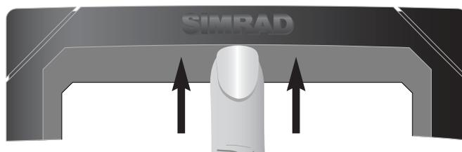
*Fig 4.4 - Removing Bezel*
