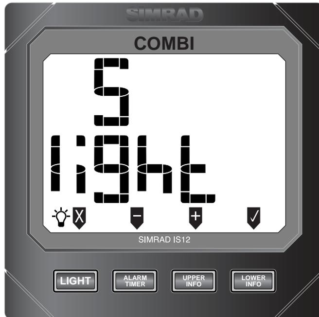
*Fig 2.11 - Adjusting Backlighting*
