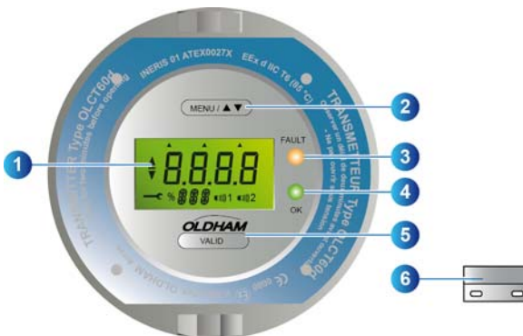
Figure 3: Detailed view of the display and its related peripheries (LED and active zones).
