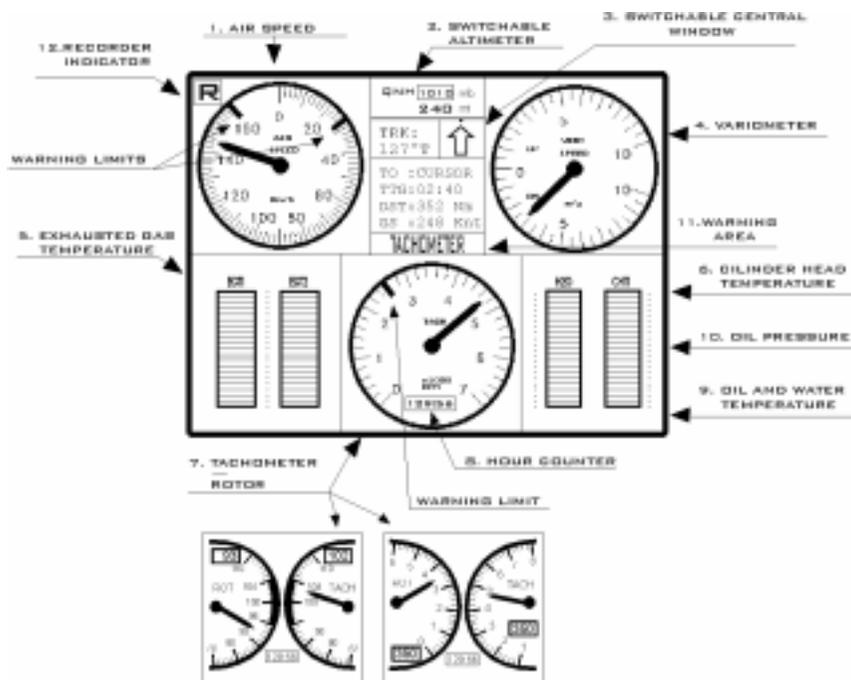
The upper part of the screen includes the flight instrumentation, the lower one engine data. We will distinguish 2 areas: flight area and engine area.
