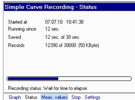
**Graphic rendering** provides a faster visual impression of the changes in the measured values. To have the measurement curve displayed while recording, select **Graph** + **OK**. The screenshot on the right shows you the curve plotted for our example.
