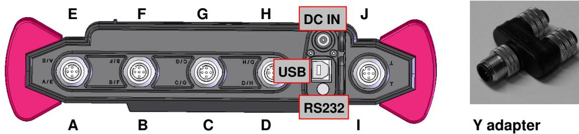
**A - E** 4 sensor input sockets\* each with two measurement channels (**channel A – D or E – H**) to connect up to 8 analogue sensors or up to 4 SMART sensors, e.g. for pressure, temperature or flow rate sensors.
