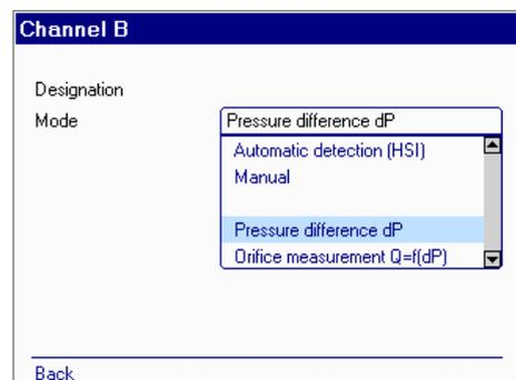
The function **Orifice measurement** **Q=f(dP)** enables you to carry out a flow rate measurement by measuring the differential pressure at a flow rate measurement orifice (e.g. HYDAC EVS 1000).
