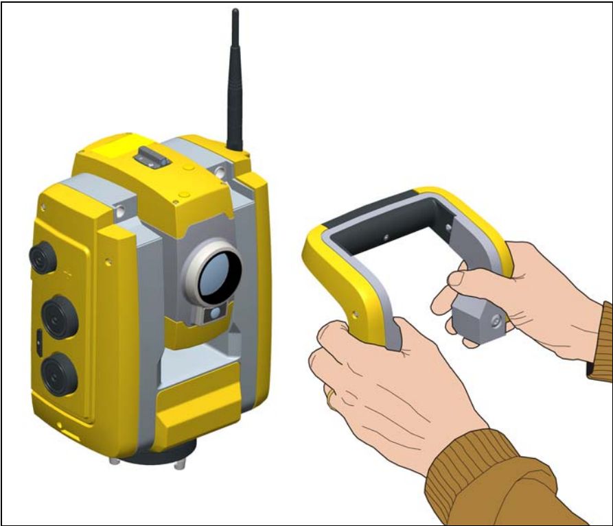
Figure 5.44 Detaching the Trimble S3 Total Station handle
