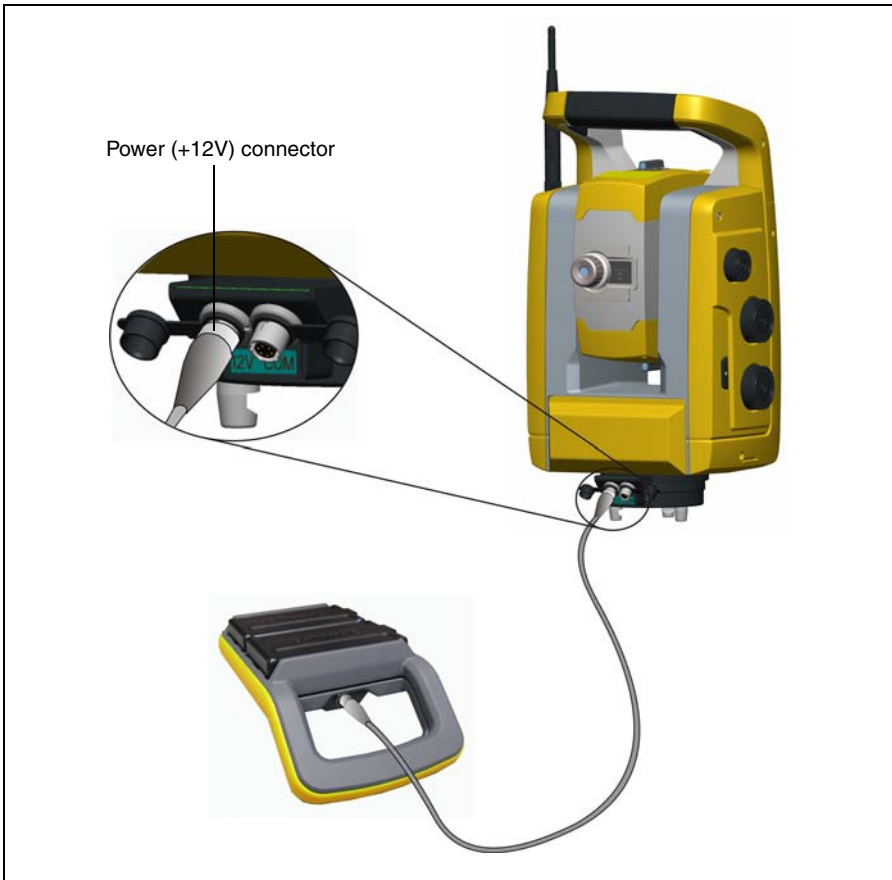
Figure 3.16 Connecting the Multi battery Adapter
