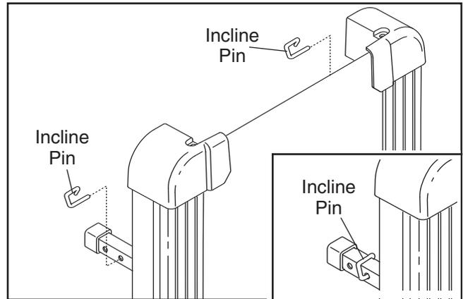
**CAUTION:** Before using the treadmill, make sure that both incline legs are at the same height. Do not use the treadmill with the incline pins removed. After you have adjusted the incline legs, lower the treadmill (see HOW TO LOWER THE TREADMILL FOR USE on page 15).
