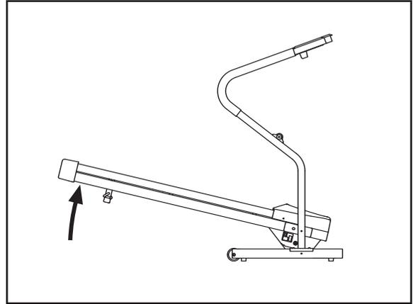
2. Move your right hand to the position shown and hold the treadmill firmly. Using your left hand, pull the lock knob to the left and hold it. Raise the treadmill until the frame passes the lock pin. Slowly release the lock knob. **Make sure that the frame is securely held by the lock pin.**
