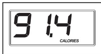
To reset the displays, press the Stop button, remove the key, and then reinsert the key.
