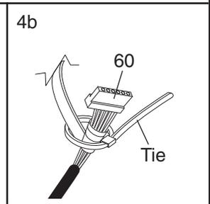
5. Carefully pull the opposite end of the tape to pull the Wire Harness (60) up through the Right Handrail (59) and out of the hole in the side of the Right Handrail.
