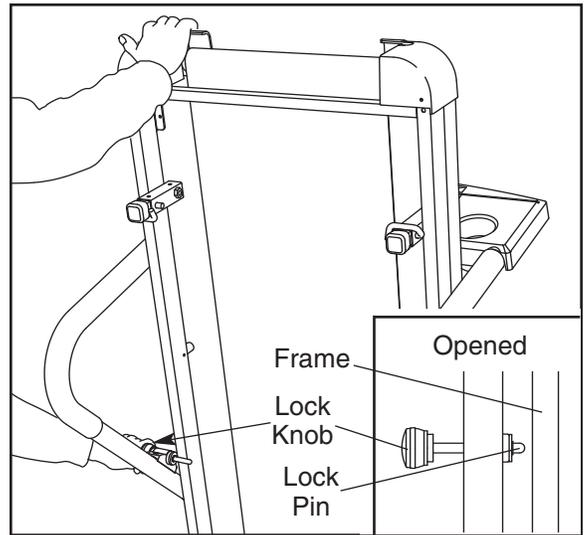
2. Hold the frame firmly with both hands, and lower the frame to the floor. **Do not drop the frame to the floor. To decrease the possibility of injury, bend your legs and keep your back straight.**
