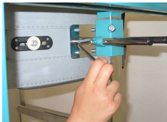
Illustration 10: Adjusting the depth of the pelvic support.
