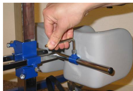
Illustration 14: Adjusting the width of the leg supports.
