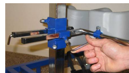
Illustration 15: Adjusting the depth of the leg supports.
