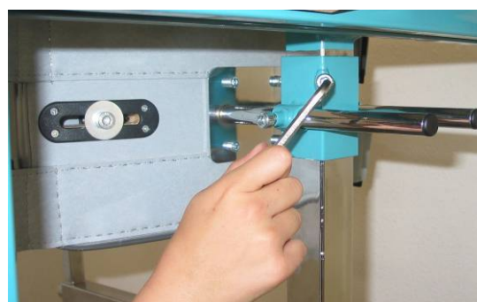
Illustration 9: Adjusting the height of the pelvic support.
