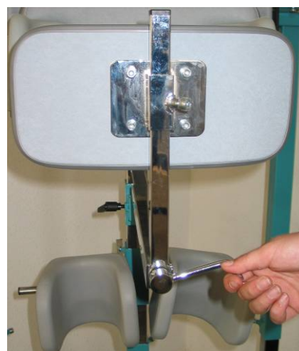
Illustration 4: Adjusting the depth of the sacral support.
