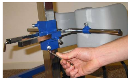
Illustration 13: Adjusting the height of the leg supports.
