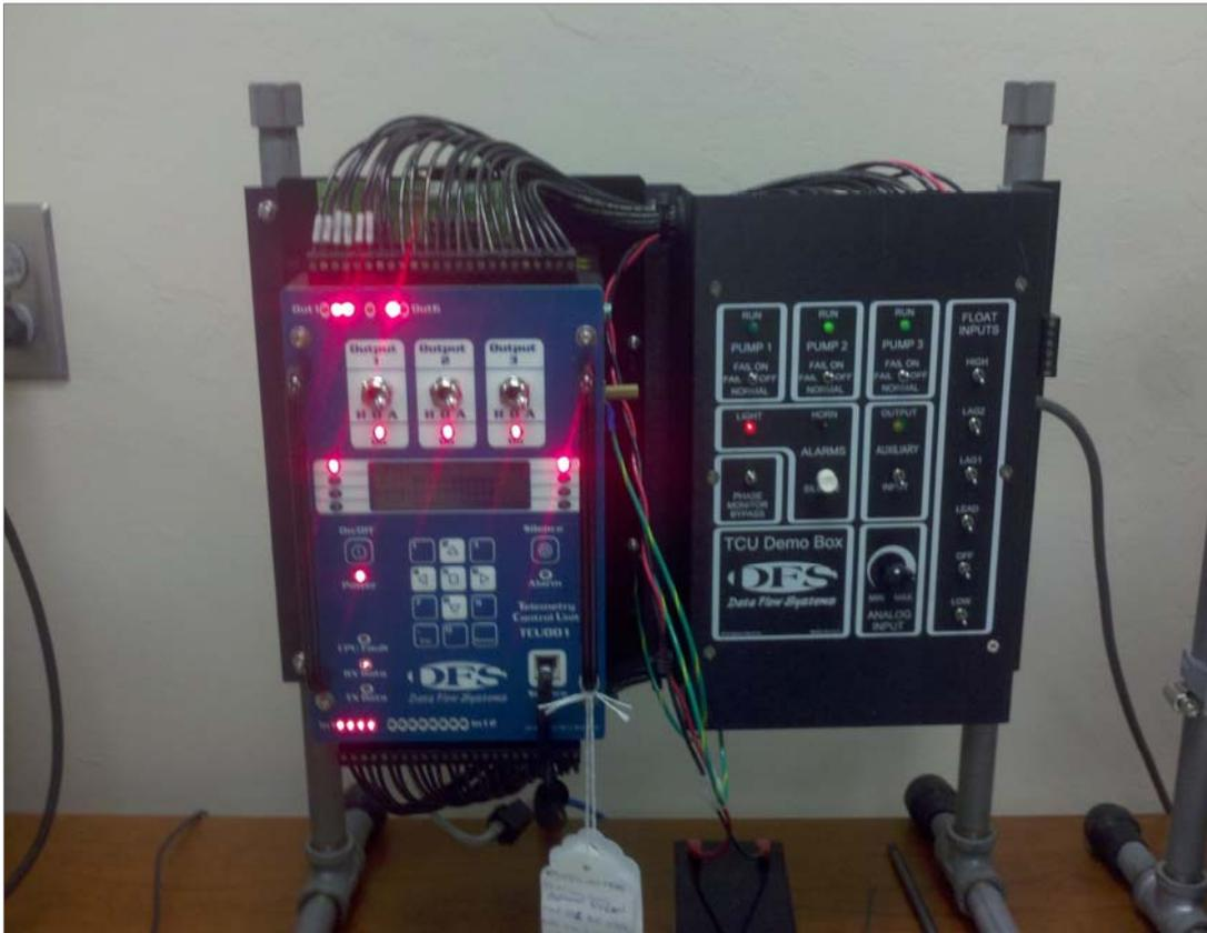
Fig. 5 Remote Terminal Unit in Florida Gulf Coast University CS lab
