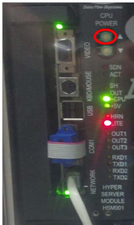
Figure 1 SCADA Server Power Up Button
