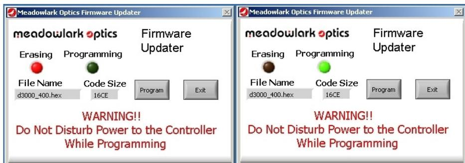
8. After programming is complete the following screen appears. When the controller power is cycled the status light should flash a pattern corresponding to the version number of the new firmware. The new firmware version may also be determined by clicking the Meadowlark Optics logo in the upper left corner of PolarVIEW.
