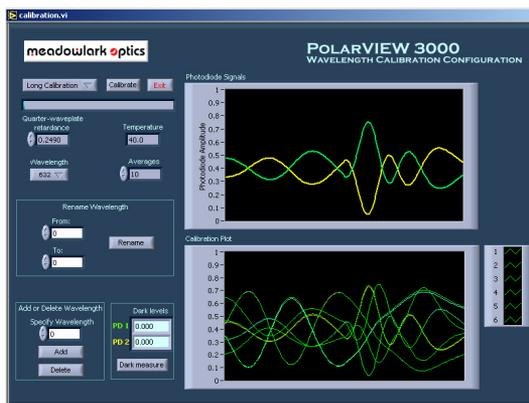
**Figure 13. PolarVIEW 3000 Wavelength Calibration Screen**
