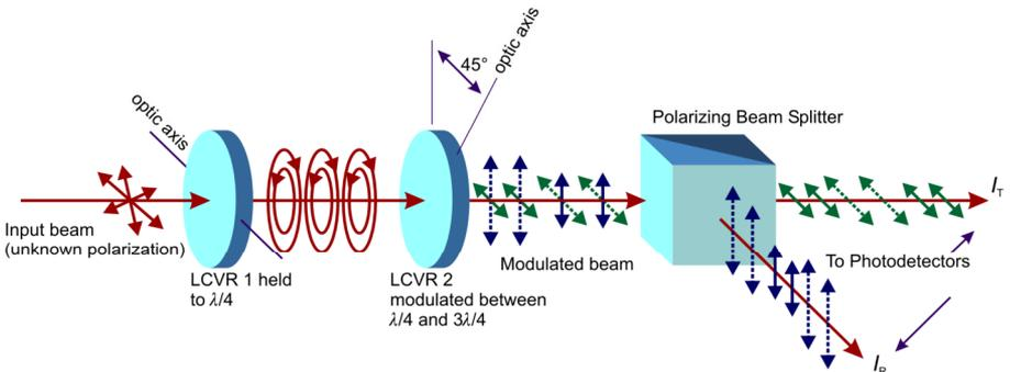
**Figure 4. Measurement of the  $S_2$ -component of the Stokes vector.**
