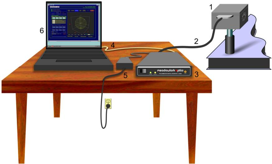
**Figure 5. Polarimeter Components.** (1) Polarimeter optical head, (2) Optical head cable, (3) D3000 Controller, (4) COMPUTER interface cable (USB), (5) Power supply, (6) COMPUTER running PolarVIEW 3000.
