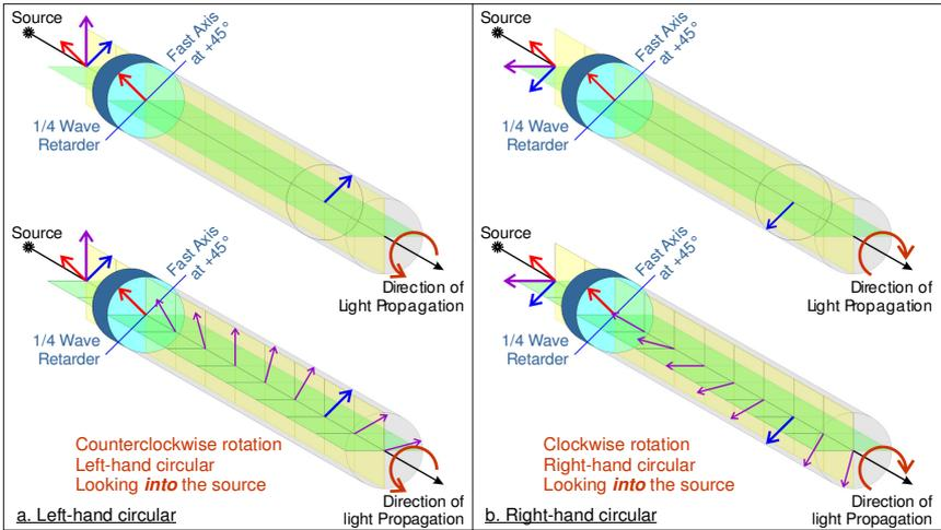
**Figure 1. Left and right circular polarization states**
