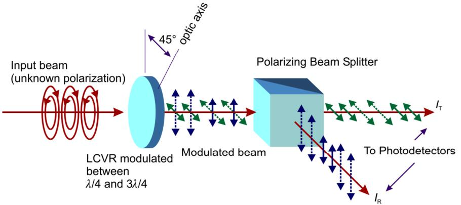
**Figure 3. Measurement of the  $S_3$ -component of the Stokes vector.**
