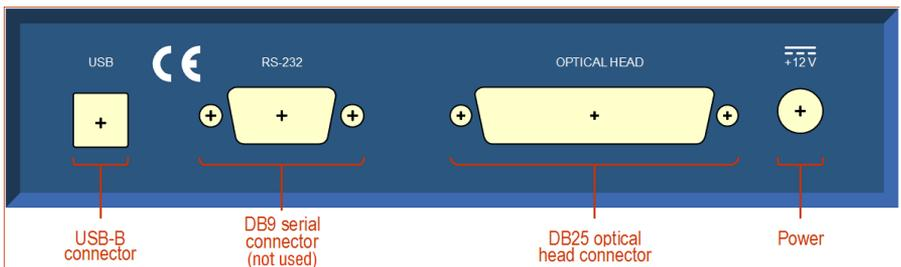
**Figure 6. D3000 connector panel**
