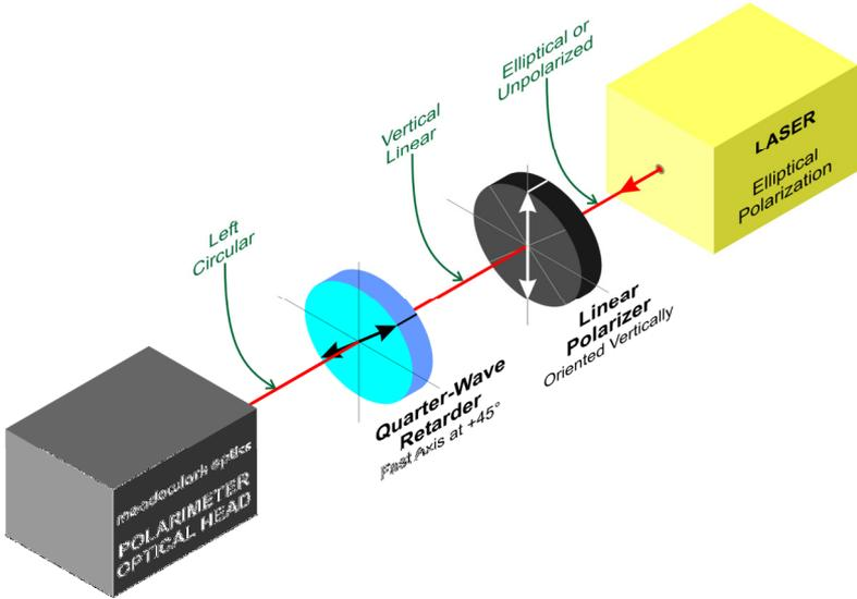
**Figure 15. Optics for Polarimeter Calibration.** The linear polarizer is rotated during the calibration procedure; the quarter-wave retarder is removed for the first four steps.
