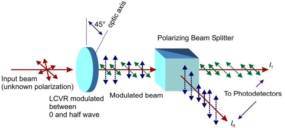
**Figure 2. Measurement of the  $S_1$ -component of the Stokes vector.**
