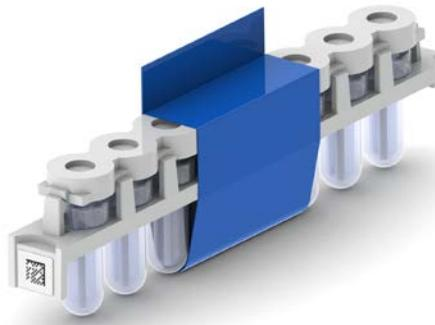
3. Load the 8 microTUBE-130 Strip (without Cap Strip) into the Cap Press Tool as shown.
