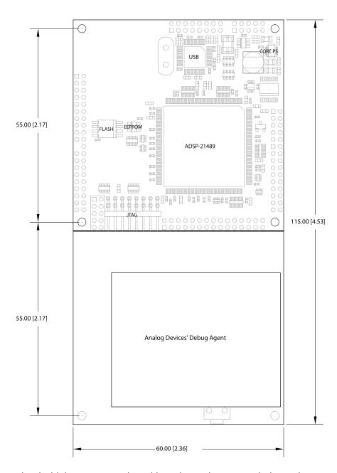
The dspblok 21489+ICE board has identical mounting holes and mating connections as the production dspblok 21489. Two additional mounting holes are provided for support as shown.
