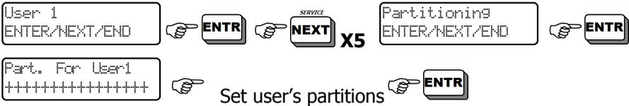
This feature links a user to a partition(s). When creating subsystems, there is also a keypad linked to each split (done by the technician), therefore the user can only arm/disarm and view the linked partition using the designated keypad. To enable a user to control his partitions from any keypad, the option "K" on the authorization bar should be set to '+'.
