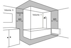
Ensure the safety zones (mm) in diagram (left hand side) are kept free.
