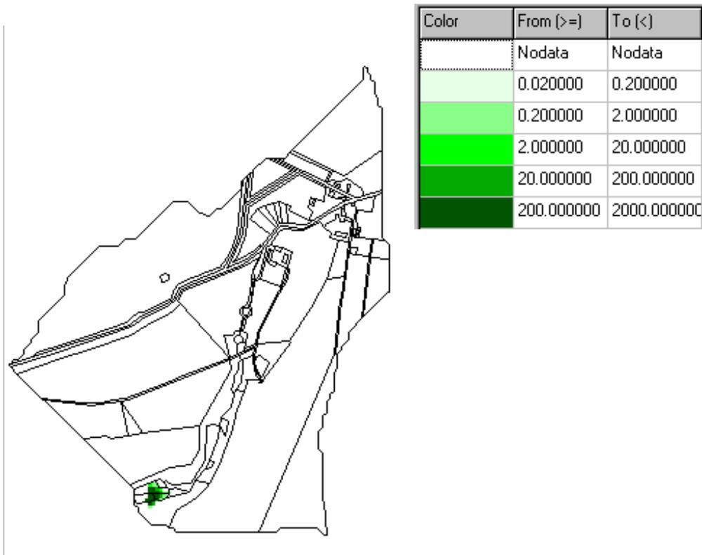
Figure 17: Deposition [kg/m<sup>2</sup>]in impoundment
