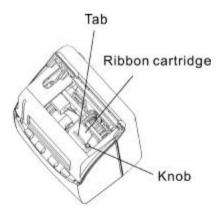
(3) Turn the knob of the new cartridge in direction of the arrow (clockwise) to tighten the ribbon.
