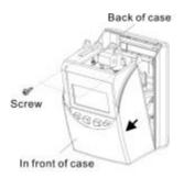
(3) Install the External time signal PC Board inside the front case. Then attach the connecting cable from the Ext. PC Board to the connector on the Main PC Board.
