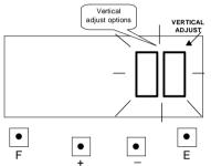
Such as example, Press the [+] or [-] button to set at "2", and then press the [E] button. At the same time, the LCD screen only display "▲" under the "VERTICAL ADJUST" mark.
