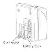
(3) Insert the battery pack into the time recorder as show in the figure.
