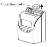
(3) Unlock with key and remove the top cover.
