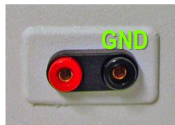
Figure 8-8: AutovaxID's Two-Pin pH Probe Connection
