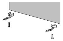
Fasten stop limit ③ through the white slide element ④ with screw
