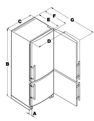
Overall height can be increased on all CS 16 units by 5/8" (16 mm) by adjusting the roller base.
