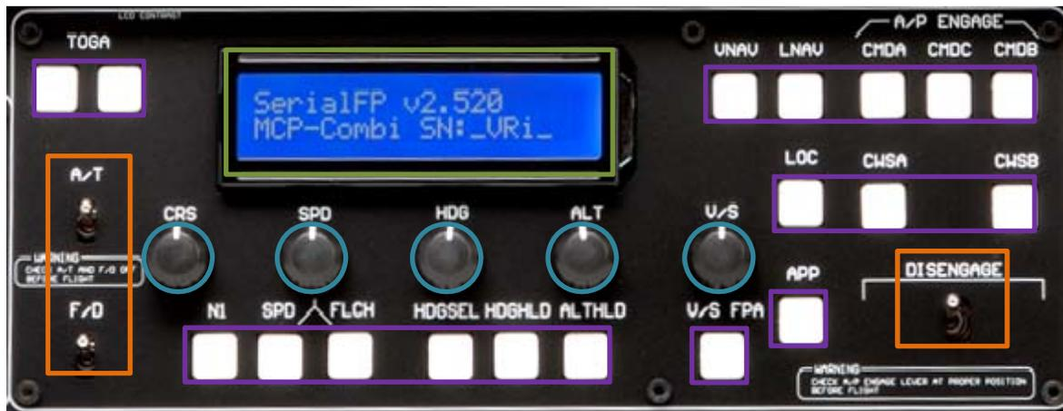
**MCP (Mode Control Panel)** : It provides control of the Autopilot, Flight Director, Altitude alert and Auto-throttle System. The MCP is used to select and activate Autopilot Flight Director System, (AFDS) modes and establish altitudes, speeds and climb/descent profiles.
