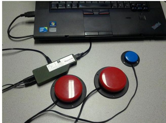
Figure 1: Connection of the switches to a Laptop Computer via the DigitalIn module
