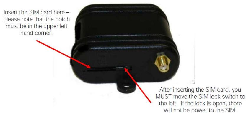
Figure 3 – Inserting the SIM Card
