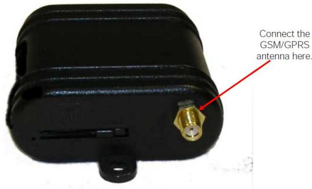
Figure 4 - Installing the GSM/GPRS Antennae
