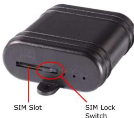
Figure 3 – Inserting the SIM Card
