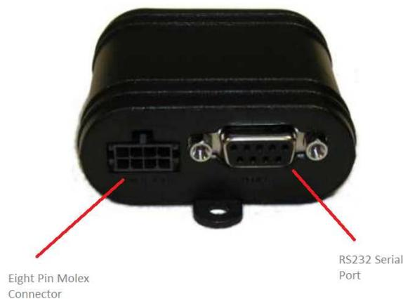
Figure 5 – Eight Pin Molex and RS232 Connectors
