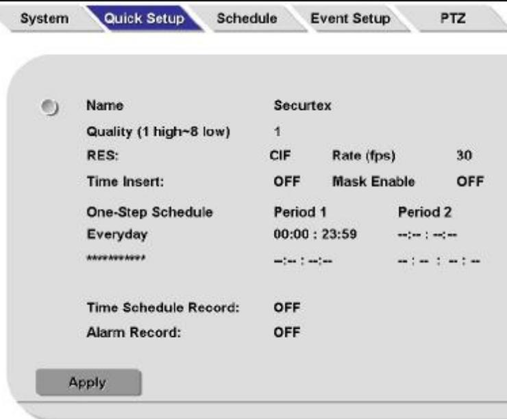
1. **Name:** select this and press "enter", then the screen will show as below. Using the remote control to move the cursor to "Back space" and press "enter" to delete the before name, then move the cursor to select and press "enter" to key-in the name. Finish to key-in and press "Apply" to confirm to setup the company name. And press the "Exit" key to back previous manual. (On Internet: directly use your PC keyboard to setup it)
