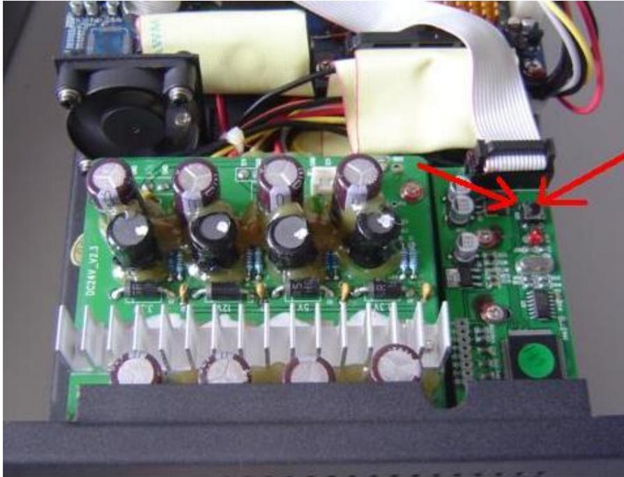
5. Within 2~3 seconds the LED light (SYS and POWER) flashing and that mean upgrading in progress; (While the LED light flashing, release the [ON/OFF] button.)
