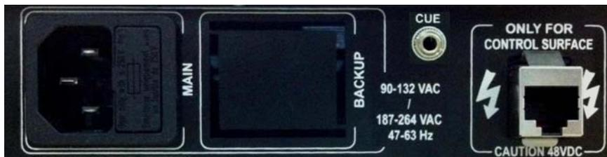
The console/engine data and power supply interconnection is located at the right of the power supply inputs. It is designed for use with straight Ethernet cabling, but also carries proprietary **power supply lines**. Please use the cable provided with the unit only. If necessary, this connection could be made by means of a cable of up to 250 meters, using a continuous CAT5E shielded (FTP) cable (or better) and checking that the screen is connected to the connectors case.
