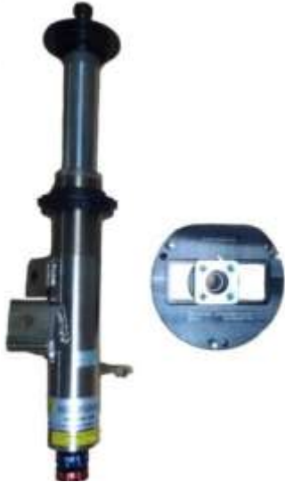
Front suspension strut incl. strut mounting
