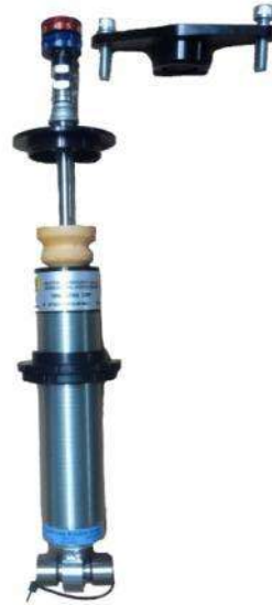
Rear suspension strut incl. strut mounting
