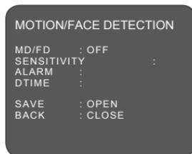
The dome camera can monitor the movement of image, and it sends an alarm message with OSD and Alarm Out action. The level for sensitivity can be changeable.
