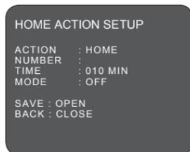
Home Action can be set so that the dome automatically goes to a preset, a tour or auto scan after the joystick control has been idle for some amount of time.
