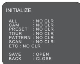
Use this function to initialize all or specific parameters of dome to factory default parameters.
