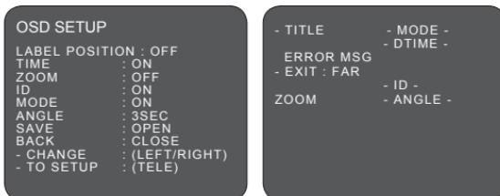
You can see only video or some character with video. Each element is able to handle. OSD setup allows you to program how labels are displayed on the monitor. Labels are such as Title, Dwell Time, Zoom ratio, Camera ID, Operation Mode and PTZ Angle. Label position can be set where you want to place on the monitor.
