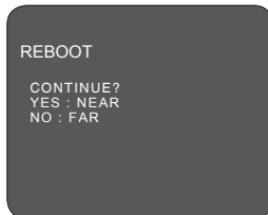
Reboot the system if there are some anomalous problems to control or operate the domes. Rebooting the system will recycle power of dome and camera without changing settings of dome.
