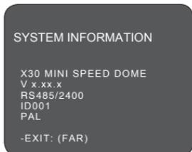
The system Information displays model name/Running Version/Protocol/Communication Type/ Camera ID No./System. It is read only for reference. Use the following steps to display the System Information screen: Camera ID changes with respect to ID switching setting
