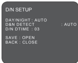
The Day & Night function improves the camera's sensitivity at night or when the brightness level of the ambient environment. According to the luminance level, Day & Night filter is automatically switched.
