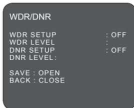
When both high-brightness subjects and low-brightness subjects have been shot at the same time, overexposure in the high-brightness subjects or loss of dark detail in the low-brightness subjects may occur. The WDR (Wide Dynamic Range) function creates images free from overexposure or loss of dark detail by combining two images after tripping the shutter for a long exposure time and for a short exposure time in one field.
