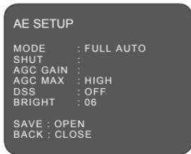
Shutter speed is the duration of the electronic shutter. Set the shutter speed to operate automatically (Auto) or manually (Numeric Value).
