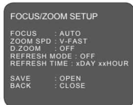
Auto Focus allows the lens to remain in focus during zoom-in, zoom-out and motion functions automatically.
