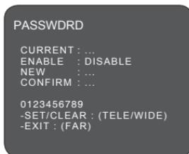
To prevent unauthorized changes to the dome settings, the dome have the feature of password protection. An unauthorized operator cannot access to any of the dome settings menus. The password must be entered before programming. The valid password with four characters must be entered to continue programming.
