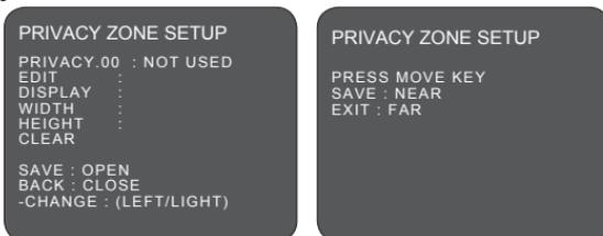
A Private mask zone allows an administrator to program one four-sided zone which cannot be viewed by operators. The mask can be changed with pan angle and tilt angle using joystick and be adjusted in size according to zoom ratio [Tele/Wide]. Maximum 15 positions can be displayed on the monitor screen. The speed of displaying masks is proportional to the number of masks on the screen. It is recommended that you set the size to at least twice the size of the object (height and width)
