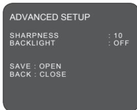
Brightness increases as the number gets higher. The backlight compensation function provides compensation by increasing the brightness of the overall screen so that subjects being shot with a loss of dark detail due to backlight will have just the right brightness level. Sharpness enhances picture detail by increasing the aperture gain of the camera and sharpening the edges in the picture.
