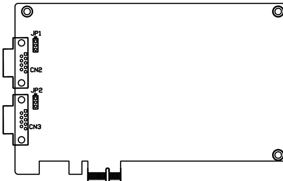
Figure 3.1 PCIE-1680 CAN-bus board silk screen
